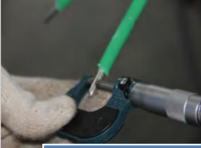
Micrometer → Outer Diameter
