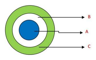
A: Solid Copper Conductor: cross section is 70mm<sup>2</sup>, diameter of the conductor is 9.4 mm-9.5 mm.
